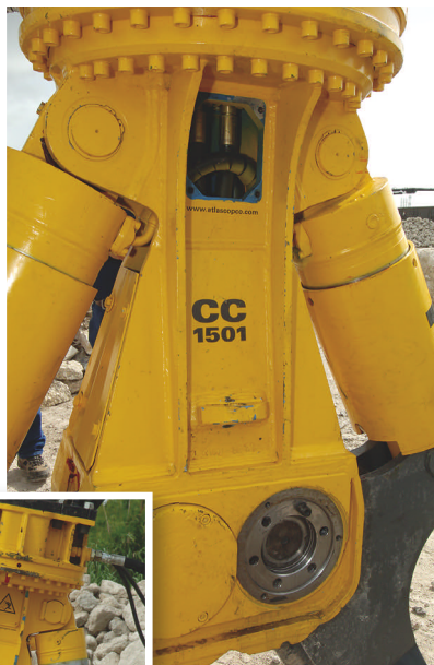
The CC 1501 uses two mounting pins to secure its jaw set to the housing (left). When the threaded pin-retainer rings are removed and the pins pulled, each of the CC 1501's jaws are freed independently and must be supported (above).
