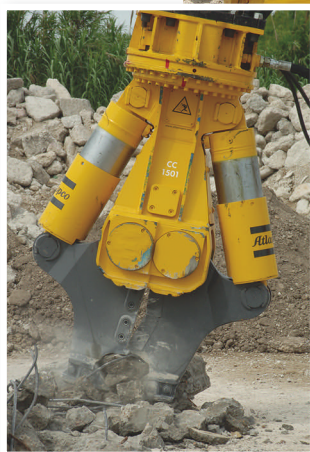
The CC 1501 uses two mounting pins to secure its jaw set to the housing (left). When the threaded pin-retainer rings are removed and the pins pulled, each of the CC 1501's jaws are freed independently and must be supported (above).
