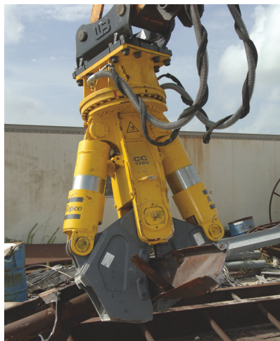
For work requiring consistent reduction of heavy-duty steel, the CC 1700's steel-cutting jaws are probably a better choice than the universal jaws.
