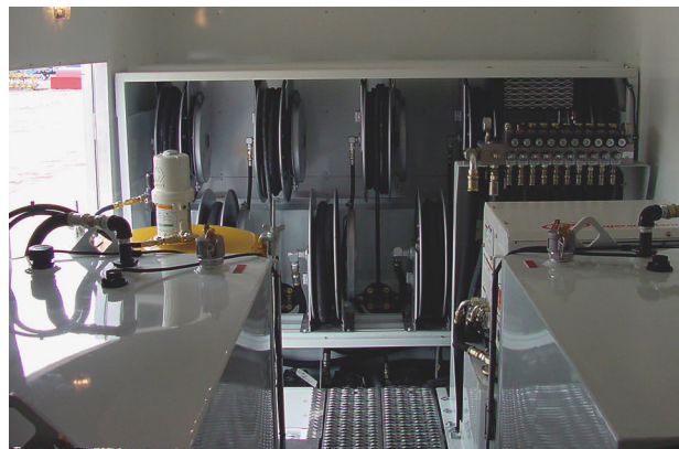
The interior of the STI Eagle Pro Lube enclosed model is bright and well lit, has tanks and sub-frame that are mounted via a spring-loaded system to resist twisting and offers a choice of air or hydraulic power for the product pumps.
