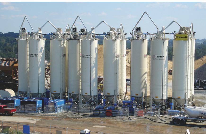
These are just a few of the silos Kiewit Southern located on site to supply paving Atlanta's Hartsfield International Airport runway addition.
