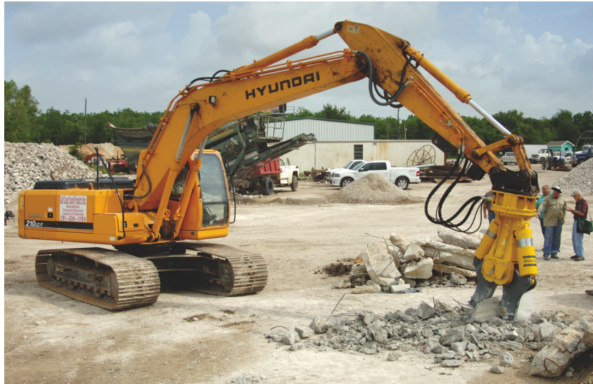
Operator Rodney Ramsey uses the CC 1501 Combi Cutter to experiment with reducing large chunks of concrete rubble in the processing yard at Gulf Coast Sand Products.
